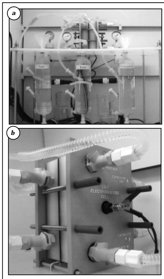
**Figure 2.** (a) Electro dialysis process system used in precious metals separation clinic project. (b) Electro dialysis cell used in the process system.
