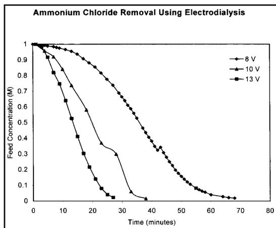
**Figure 3.** Typical student data showing the effect of voltage on the removal of an ammonium chloride contaminant from a precious metal feed solution.
