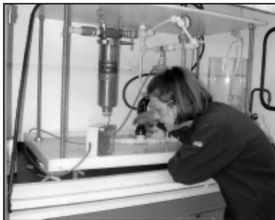
**Figure 1.** Student conducting membrane separation study of vegetable product stream.
